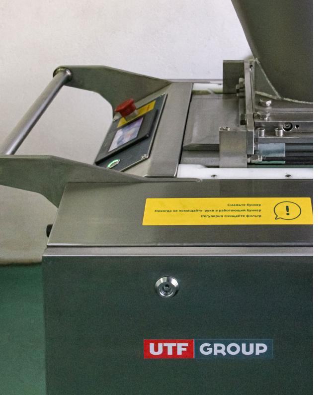
Quick change of types of dough, as it does not remain in the vacuum chamber, which together with the fastening of the hopper 4 bolts for easy and quick cleaning of work surfaces
